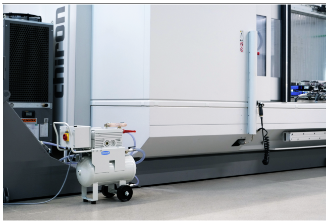
Vacuum unit VAGG for vacuum generation on a CNC machining center
